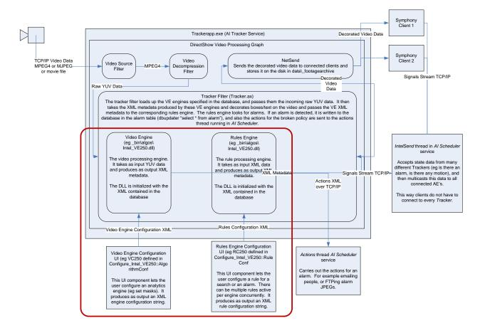
A user configures the analytics and rule engines using corresponding *C# analytic and rule configuration UI components*. These components are plugins for Symphony. They should be deployed into the Symphony Server's \_bin\algos folder. Symphony Client pulls the UI plugins from the server when needed. Configurations are saved as XML in the database. The configuration strings are used to initialize the analytic and rule engines when the AI Tracker Service starts.
